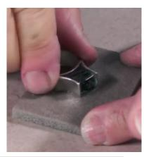
use sand paper, change it between grits to keep stray particles from scratching the resin.
